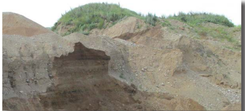
A bad example of taking material from a narrow area of the working face of a gravel bank not allowing good blending of material.
