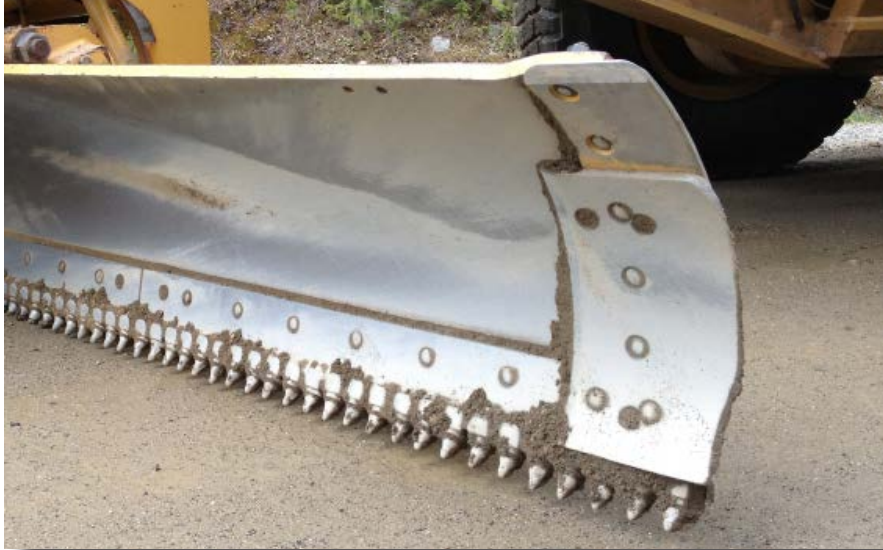
An excellent tool for preparing loosening and preparing a road surface is a moldboard cutting edge equipped with carbide bits.
