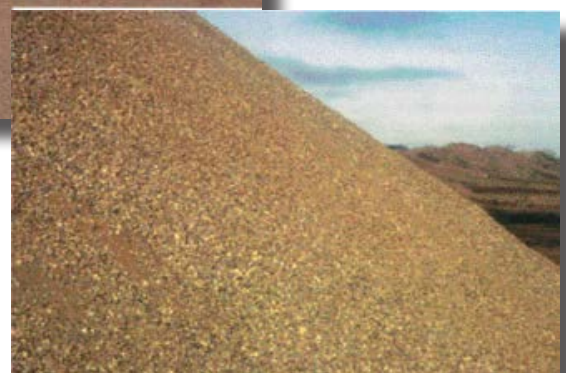
...while the back side (seen here) has excess stone. This could have been prevented by eliminating segregation on the stacker belt.
