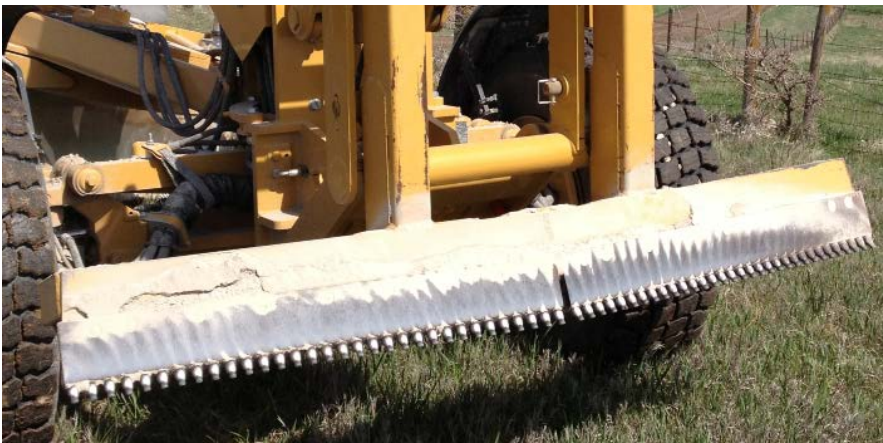
A cutting edge with carbide bits is effective to loosen washboard areas.
